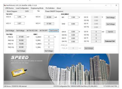
**POINT OF ATTENTION.** On this page you can set the SHD pin. With this digital pin high (SHD=3.3V) the TIAs are working. With 0V the TIAs are shutdown.
