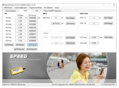
• After setting the VOA to 4V (all the PDs show significant current):
