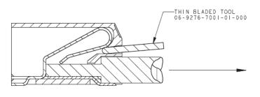
PUSH BLADE (NOT SHARP) INTO SLOT ABOVE WIRE. WHEN WIRE IS FREE, PULL TO EXTRACT.
