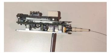
The intent of the design is to insert a screw through the shield into the standoff. That would stabilize the configuration for long term operation. However, so far we only have found 1/8 screws which do not fit between the shield and the board. So this is not ideal.
