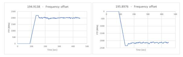
We monitor the output to the PZT through the register 0xFD with datafield 0x9001 (read operation). We can see that the PZT is working hard to keep the signal close to the target. Most importantly the correction signal stays within the range of the control (0-65535) and does not rail.
