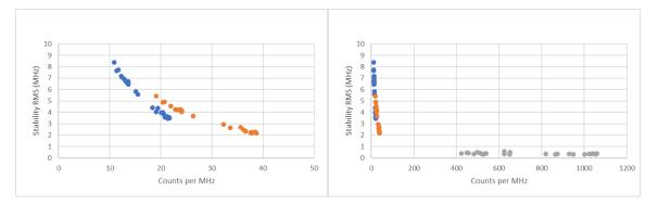
For further reference, the data for our PPCL590 is included in the second graph so show capabilities with higher resolution. Also, it likely shows that beyond 150 counts per MHz other effects are limiting the frequency stability that can be realized.
