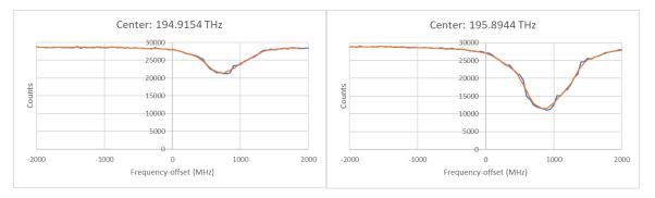
We process such data by averaging and finding the frequency offset points (X, Y) where the absorption is half of the max absorption. We also determine the slope (in counts/MHz) at those points. That data allows us to determine at each peak:
