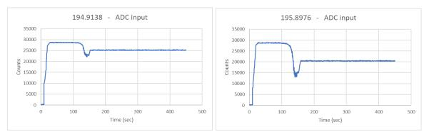
We monitor the FTF value through register 0x62. On the left hand slope, The device starts 2000MHz below the target value and moves up in frequency until it locks. On the right hand slope the device starts 2000MHz above the target value and moves down. After stabilization you can see the FTF value moving around, to ensure that the feedback signal to the PZT remains centered.
