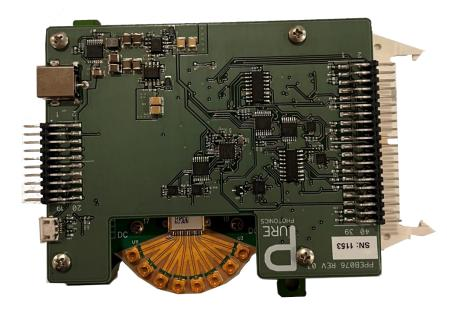
Add the 40pin IDC cable. For <u>PPEB076 rev4/PPEB086 rev3</u> there is no need for a ribbon cable. If a ribbon cable is desired to be used, then plug it on the top connector of the PPEB076 rev4.
