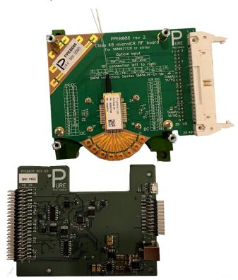
Mount the PPEB076 on top and align the holes with the standoffs. Insert the M3 screws into the standoffs. The 40pin connectors should be on the same side. For <u>PPEB076 rev4</u>, the 40 pin connector on top of the PPEB086 will align with the 40pin connector on the bottom of the PPEB076. Push these connectors together. For connecting a <u>PPEB076 rev3 to a PPEB086 rev3</u>, make sure the ribbon cable is inserted before inserting the M3 screws.
