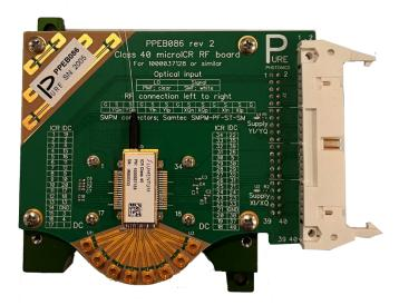
After completion the assembly should look as above (rev2). The rev3 looks the same, but the board is less wide and the connector is between the two left M3 screws.
