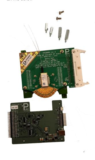
Remove the 2 M3 screws in the upper corners of the PPEB086 (making the total number of screws 4), Replace them by the 14mm stand-offs. Add the 20 mm standoffs in the open M3 holes
