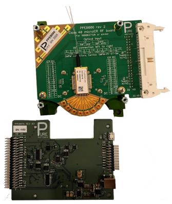
Mount the PPEB076 on top and align the holes with the standoffs. Insert the M3 screws into the standoffs. The 40pin connectors should be on the same side.
